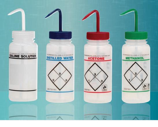
These 500ml wash bottles ensure leak-proof dispensing of your most common solvents in the laboratory. Easy-to-read, LDPE solvent-resistant printed bottles include: DOT and NFPA codes and symbols, CAS numbers, protective equipment symbols and target organ information making your laboratory a safer place. Each bottle includes color-coded cap with wash tube.
