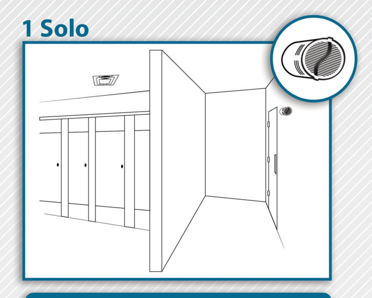
The unit is installed near the door opposite the hinges, because this door opens inwards. The "air-in" vents are above the restroom stalls which will pull the fragrance across the restroom maximizing performance and coverage.
