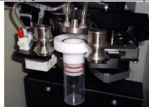
Visually verify that the Filter has been properly loaded into the instrument.
