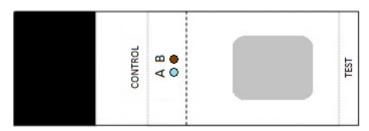
Slides are designed to be used as same-slide. Test sample should be placed below the control, in the area marked 'TEST' (see diagram above).
