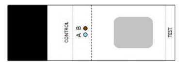
Slides are designed to be used as same-slide. Test sample should be placed below the control, in the area marked 'TEST' (see diagram above).
