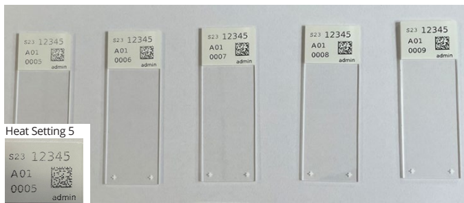
Superfrost Plus starting with heat setting 5 on the left, to heat setting 9 on the right
