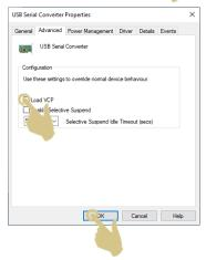
1.1.10. Check again for the com port and note the number – in this example, the com port is COM7
